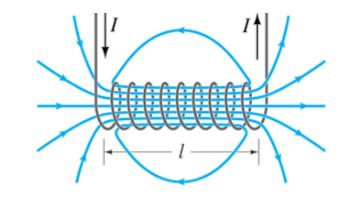
The right-hand grip rule can be used to find the direction for the magnetic field.
