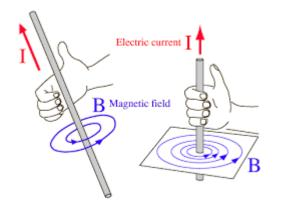
For single wires - Point your thumb in the direction of the current. The direction of your fingers shows the direction of the magnetic field.
