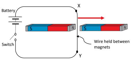
Closing the switch creates a force that acts on the wire XY.
