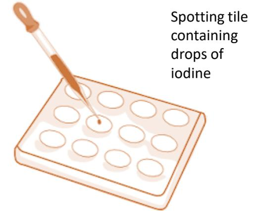
Starch reacts with amylase in a water bath. Samples are taken from the mixture every 30 seconds and added to the iodine in the spotting tile. Iodine goes black = starch present – this happens when starch has not been digested yet or if the pH is too low or too high. Iodine stays brown = no starch present (the starch has been digested). The quicker it remains brown, the faster the rate of reaction. This will happen at pH 7-9. This is repeated for a range of different pH solutions.
